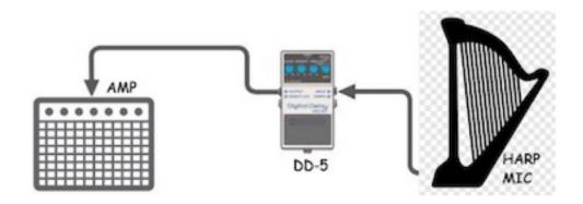
take a cord from the pickup on your harp into the right side of the delay pedal IN, then a cord OUT from the left side of the pedal into the input on your amp. It's that simple.
